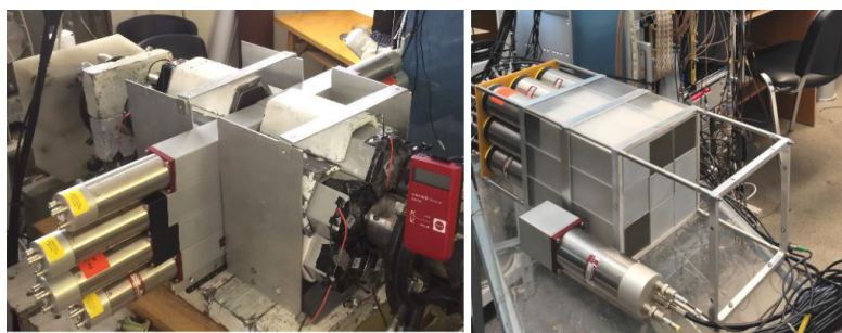
Figure 1: (Left) 8 phoswich detectors coupled to 12 CsI(Tl) 4 \pi \gamma -spectrometer. (Right) Cluster of 9 phoswich detectors.
