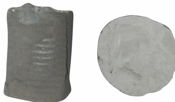
Fig.2. Picture of the nitrated mixture of aluminum ferrosilicon, marshalite, nitrated product, and ammonium fluoride.
