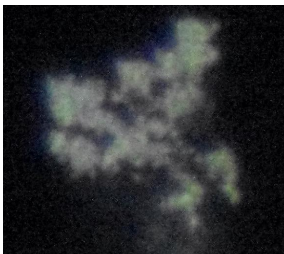
Fig.1. The erosion traces leaved by five low current short-term discharges (10mks,4A)
