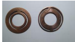
Figure 2- Split rings printed and copper plated
