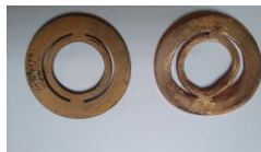
Figure 3- Split rings printed copper plated with sputtering technique
