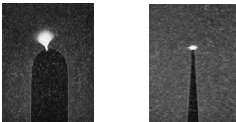
Fig.3. Typical images of corona glow on the cathodes of different diameters. L. B. Loeb, Electrical Coronas , Univ. of California Press, Berkley, USA (1965)
