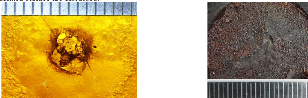
Fig.1. A sample of igdantin (left) and rubber (right) after exposure to an electron beam with an energy of 580-600 J.
