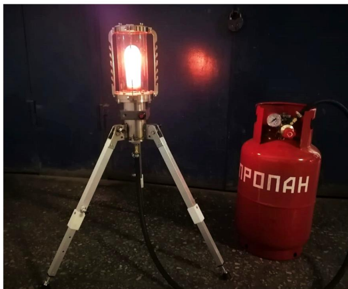
Fig.1. Image of IR heater based on self-aspirated radiant burner operated in the internal combustion mode.
