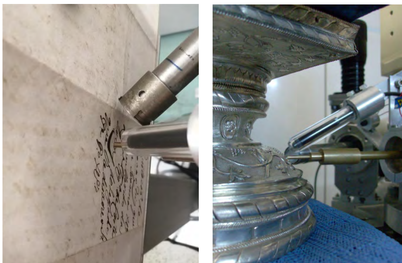
FIG. 1. Different type of materials (paper with iron-gall ink and metallic object) during the measurements in open-air conditions.
