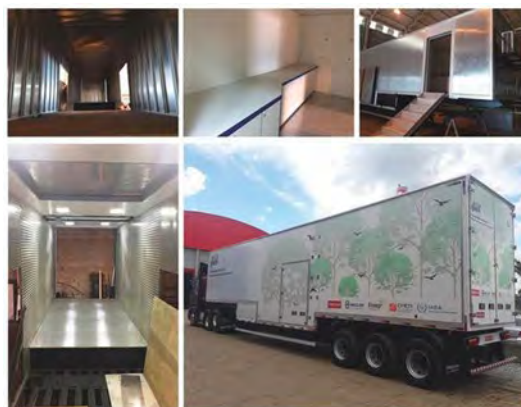
FIG. 1: Mobile electron beam irradiation unit for the treatment of industrial effluents in Brazil.
