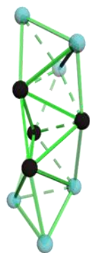
Fig. 1. Tetrahedrally tightly packed spiral in the structure Al_4C_3
