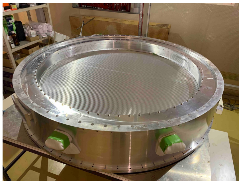
Figure 8. Photograph of the straw tracker being assembled (first station).
