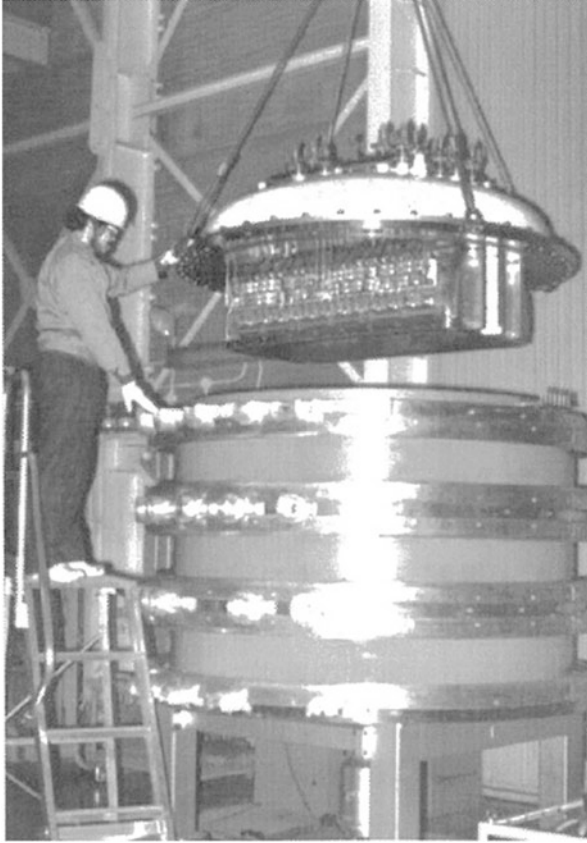
Fig. 19.10 Assembly of the large negative ion source, extractor, and 500 keV electrostatic accelerator for JT-60 U negative-ion-based NBI
