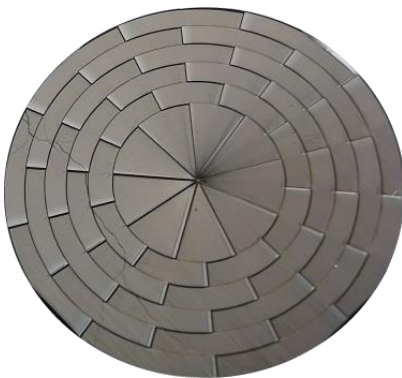
Fig.1. Optical image of the fabricated diamond axicon.
