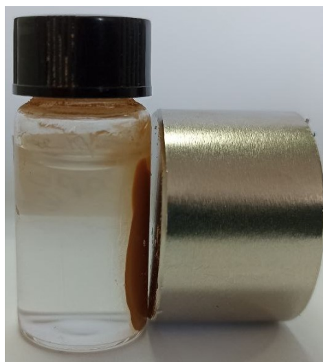
Fig. 2. Immobilisation of magnetic polymer microspheres by the influence of permanent magnet of 8.62 kg
