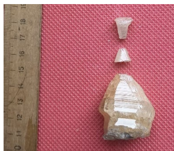
Fig. 1. Li_x Mo_y O_z crystal grown by LTG Cz technique
