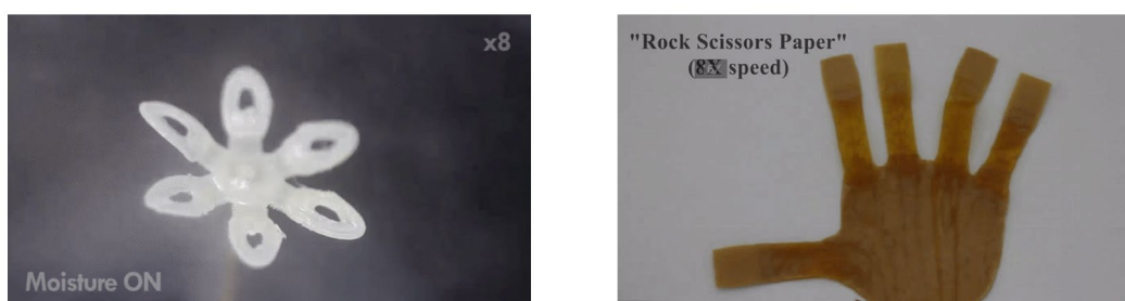
Fig. 1. Liquid crystal elastomer-based hygroscopic actuator (left) and artificial muscle (right)
