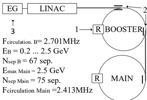
Fig.1. 1 — Rezonator; 2 — Kiker; 3 — Electron gun.
