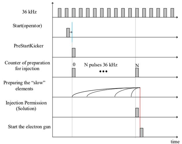
Fig. 3. Graphical representation of the signals when electron bunch injecting from Linac to Booster.
