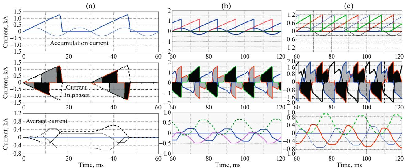
Fig. 4. Curves of accumulation currents, total currents by phases (each phase is highlighted in its own color), and average currents in each phase of the power supply for (a) one, (b) two, and (c) three modulators. In the upper figures, a sinusoid of the mains voltage (50 Hz) is shown for clarification.
