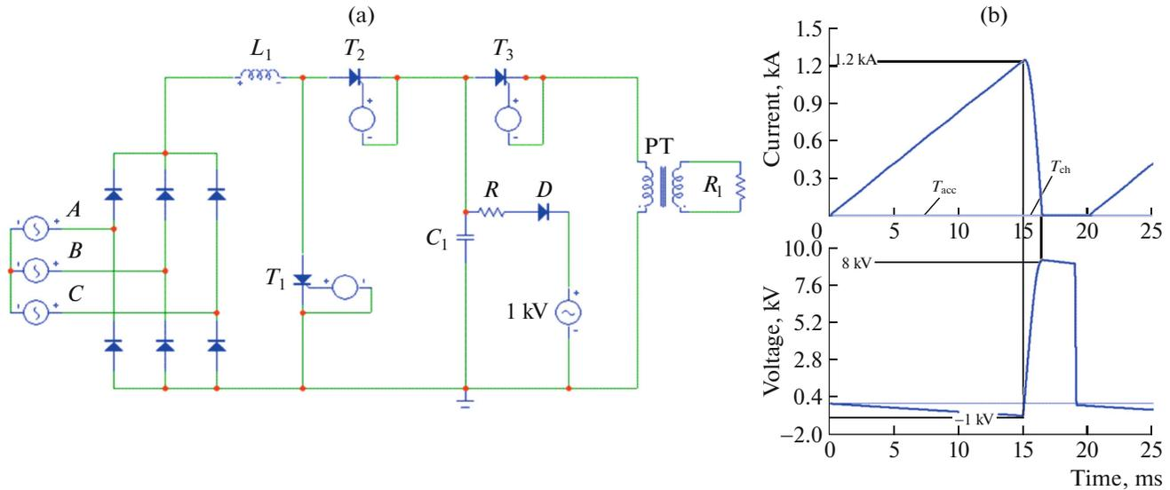
**Fig. 1.** (a) Scheme of pulsed current accumulation in the inductance and charging of the capacitance of the forming line ( $T_1$ – $T_3$  is synchronized switch assemblies; PT is pulse transformer); (b) timing diagrams explaining the operation of the modulator.
