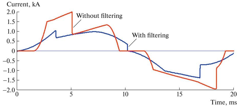
Fig. 5. Influence of filtering chokes on the shape of the period of phase *A* current.
