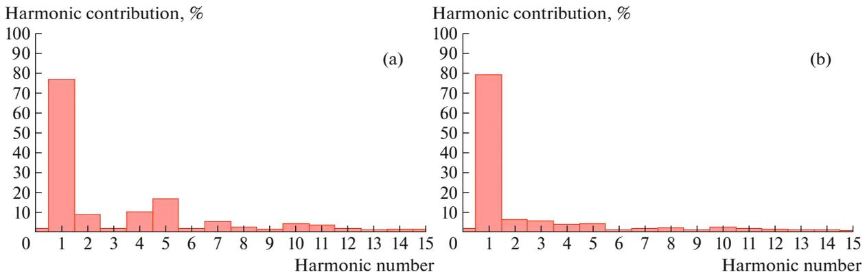
Fig. 6. Phase *A* current expansion in terms of harmonics: (a) without additional inductances and (b) with filter chokes.
