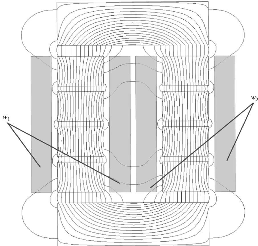
Fig. 2. Estimated picture of the distribution of the magnetic flux along the magnetic circuit of the modulator accumulation inductor.
