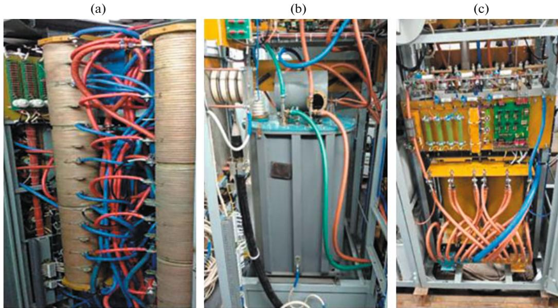
Fig. 3. Cupboard: (a) with forming line  $C_1$ ; (b) with pulse transformer; (c) with accumulative choke  $L_1$ .
