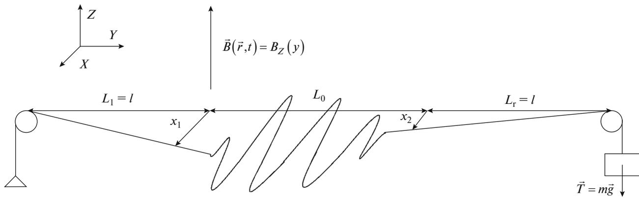
**Fig. 1.** Scheme of the measuring system. If the magnetic field has only vertical component  $B_z$  and there is no wire sag, the wire is curved only in horizontal plane  $XY$ .
