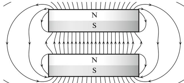
**Fig. 2.** Magnetic field lines of a pair of coils without allowing for the magnetic conductor.
