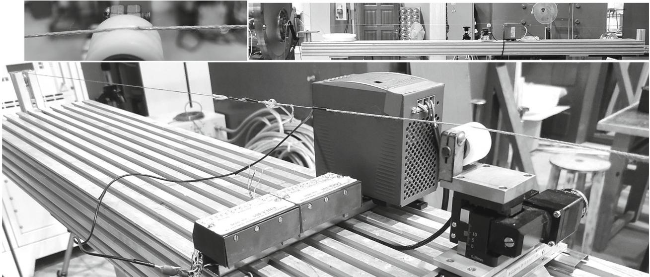
**Fig. 3.** Scheme of stretching a composite wire. A current-carrying copper cable emerges from a Kevlar sheath between the rollers. The roller on the motorized transport modules experiences a minimal load.
