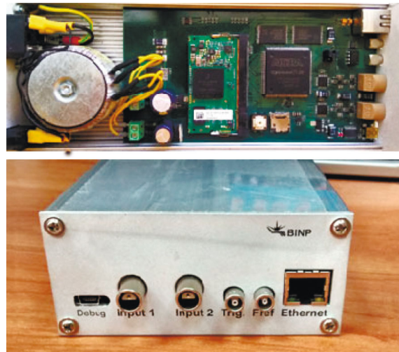
Fig. 13. Photographs of the measurement module of the dispersion interferometer.
