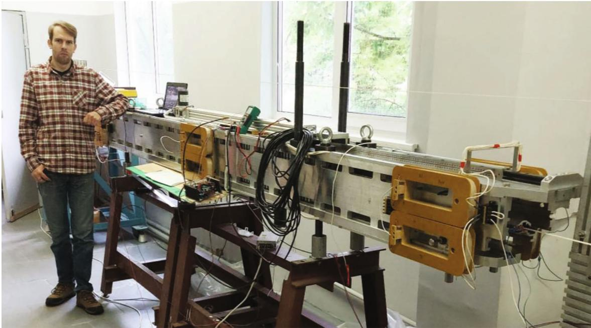
**Fig. 2.** Photo of the undulator installed on the stand for magnetic measurements. Magnetic field correction windings are visible in the middle and at the ends of the undulator.
