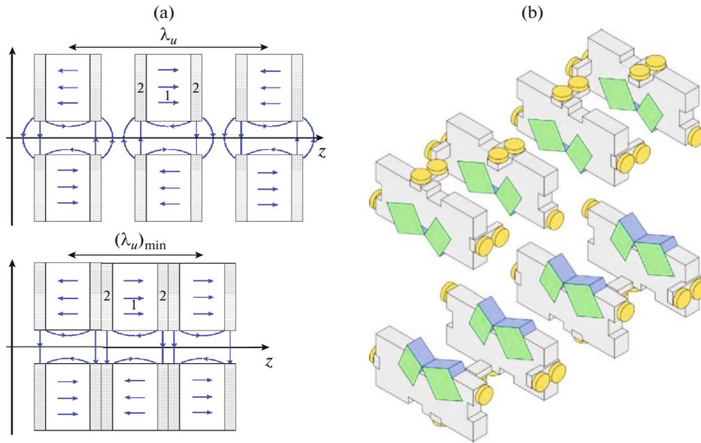
**Fig. 1.** (a) General scheme of an undulator with a variable period for two different periods: (1) permanent magnet and (2) iron plate. Blue arrows show the direction of magnetic induction. (b) 3D model and arrangement of cassettes. Blue shows permanent magnets, green shows iron pole strips, yellow shows ball bearings, and gray shows aluminum cassette housings.
