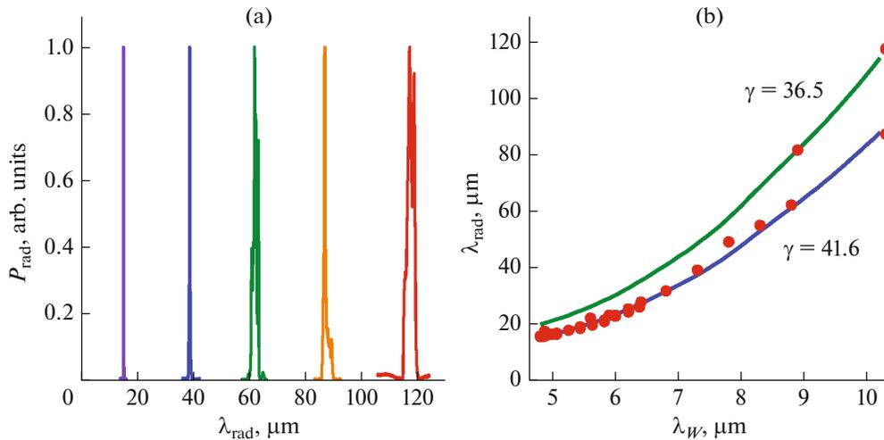
**Fig. 3.** Measured emission spectra in different regions of the tuning range (a) and measured dependence of the wavelength on the period of the undulator (b). The solid line shows the theoretical dependence of the wavelength on the period for two different electron energies.
