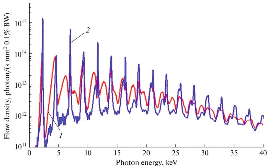
**Fig. 2.** Emission spectra calculated by the SPECTRA program based on the uncorrected (1) and corrected magnetic field (2) of the undulator.
