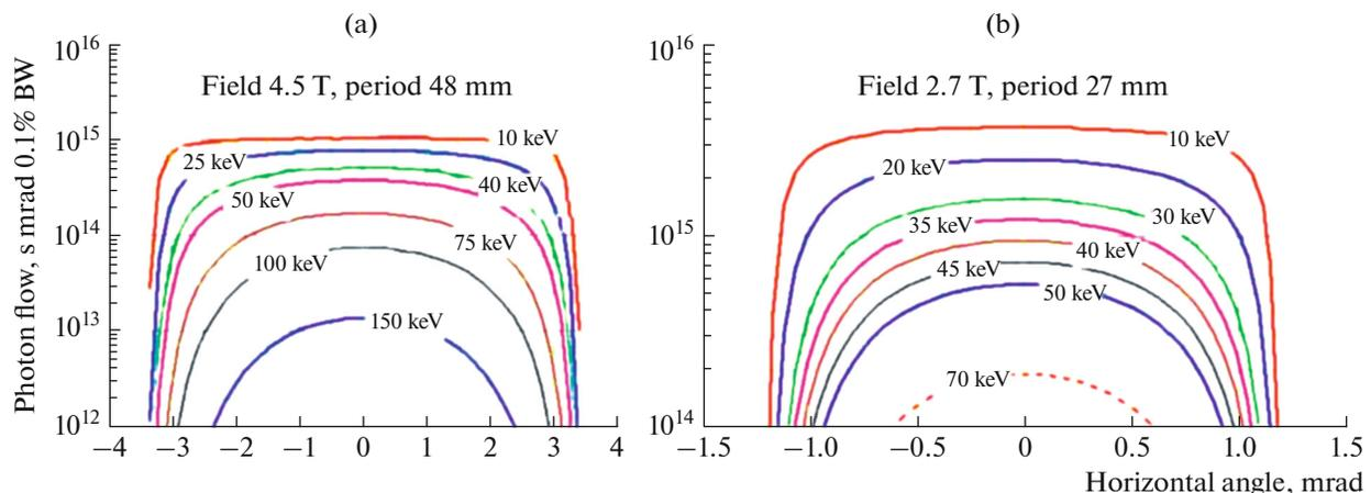
**Fig. 1.** Spectral-angular distribution of the photon flux from wigglers with a field: (a) 4.5 and (b) 2.7 T.
