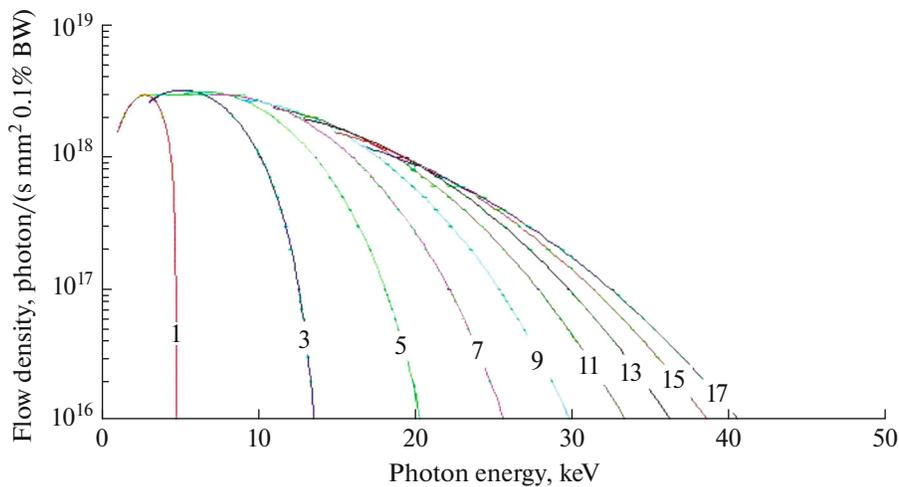
**Fig. 3.** Spectral flux of photons at harmonics from 1 to 17 when the field changes from 0 to 1.6 T.
