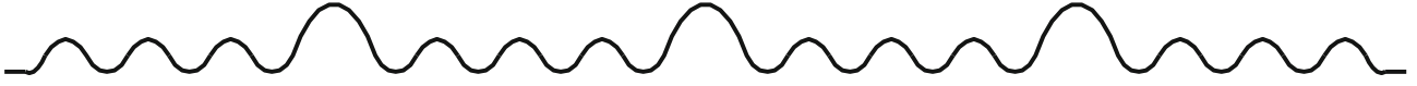
Fig. 1. Electron trajectory in DOK with M = 4 undulator sections and M - 1 = 3 chicanes. Number of periods at each undulator is N_1 = 3 .
