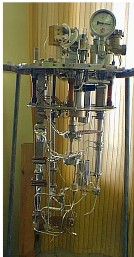
Figure 2. Cryostat for 4 K cooling of 3 mm SIS mixer receiver RT-22 Simeiz telescope.
