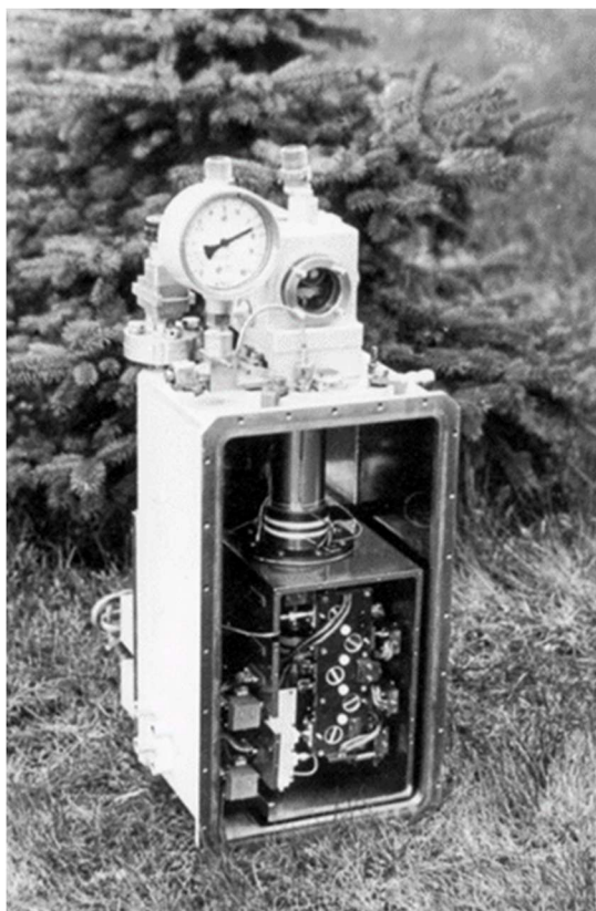
Figure 1. Cryostat for 20K cooling of Shottky Barrier Diode 4 mm receiver (the 1-st!) RT-22.
