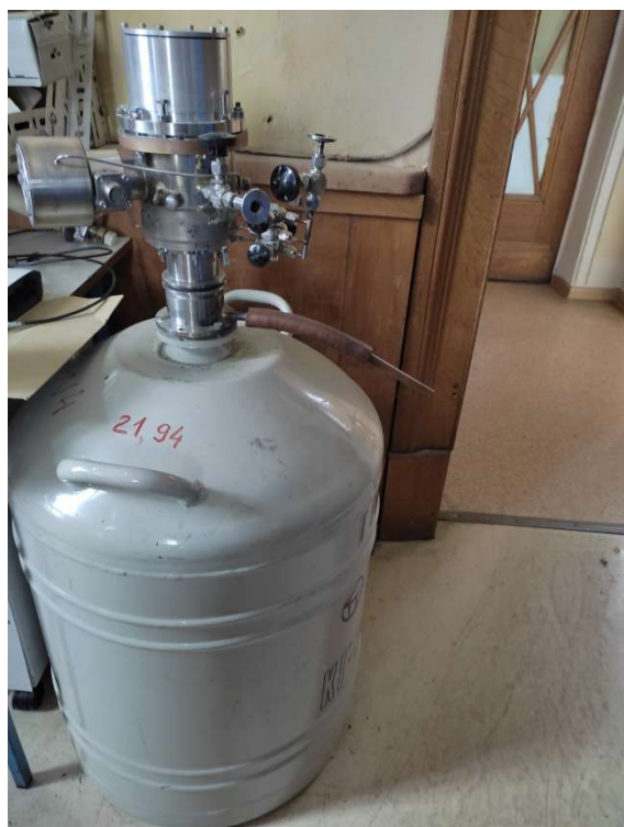
Figure 7. Dilution subK L3He-4He cryosystem (deep stick).
