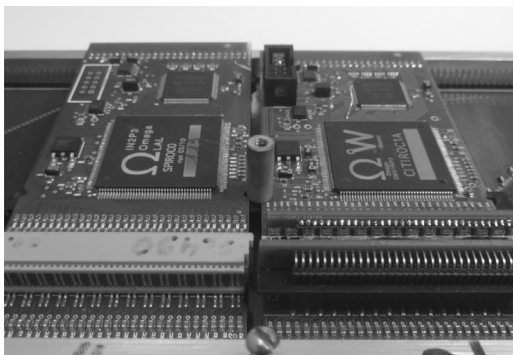
Fig. 3. General design of detector boards with KETEK and HAMAMATSU micropixel photon counters (left) and pulses at outputs of ASIC fast shaper (right).
