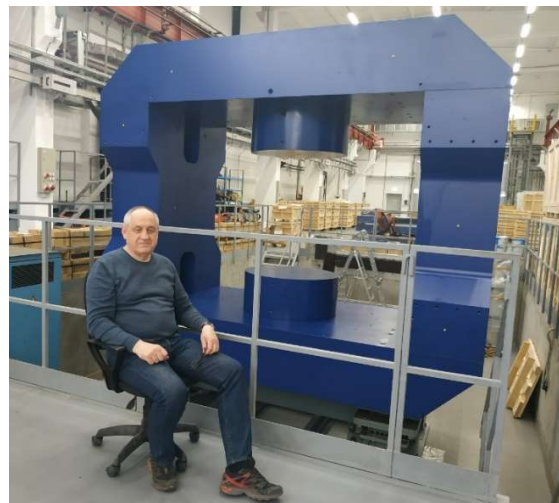
Fig. 10. The view of the assembled iron yoke on the test place in BINP.
