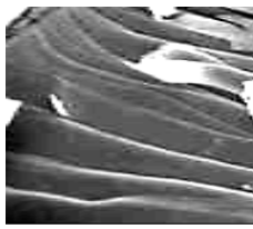
Fig.2. Layered, textured microstructure of the Bi/Pb cuprate and ferroelectric has used for mix systems preparation
