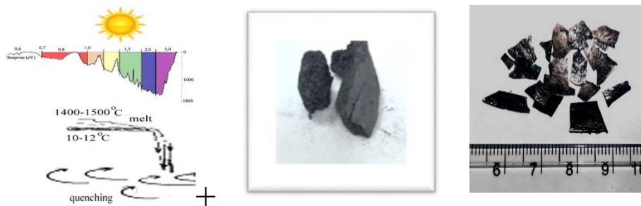
Fig.1. Sheme of the technological process in the Large Solar Furnace (Parkent) and the precursors
