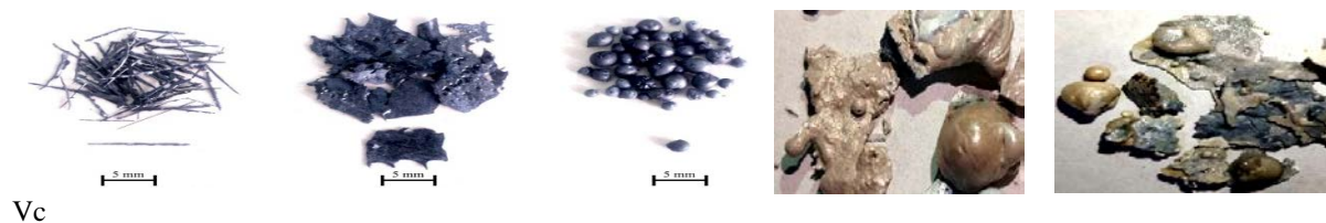
Fig.1. Bi/Pbcuprate and \text{SrTiO}_3 , \text{BaTiO}_3 synthesized in Larg Solar Furnace (Parkent) for mixed system preparation.
