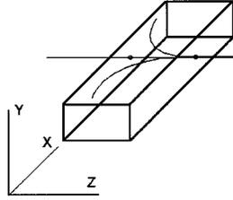
Fig. 2. – Schematic drawing of the proposed experiment. The electron beam passes through the holes in the wave guide located at a node of the standing wave. For the field magnitude larger than some critical value this trajectory becomes unstable and electrons scatter randomly.
