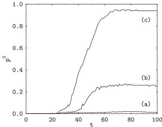
Fig. 3. – Chaotic diffusion of the momentum for the electron beam injected in the wave guide at a node of the standing wave: (a)  $\kappa = 1.5$ ; (b)  $\kappa = 1.8$ ; (c)  $\kappa = 2$ .
