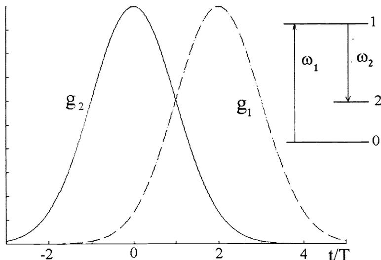
Fig.1. A configuration of energy levels in atom and Rabi frequencies at an input of a medium.  $\omega_{1,2}$  — carrier frequencies of probe  $g_1(t)$  and coupling  $g_2(t)$  pulses, consequently.
