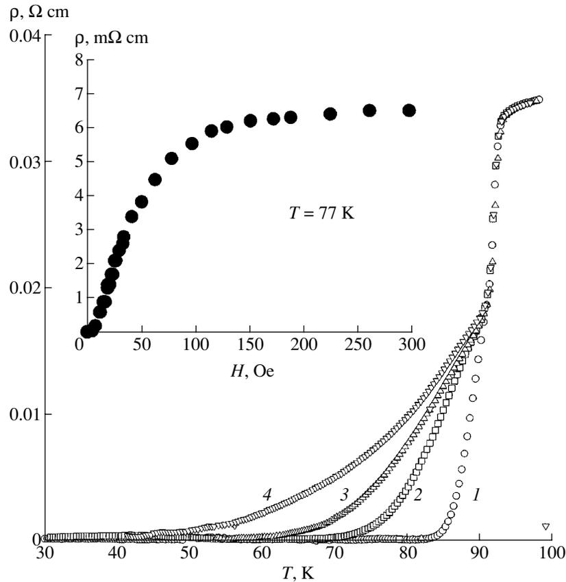
**Fig. 1.** Temperature dependences of the resistivity  $\rho$  of a 85 vol % YBCO + 15 vol % BaPbO<sub>3</sub> composite measured at various values of the applied magnetic field strength  $H = 0$  (1), 38 (2), 79 (3), and 270 Oe (4) using a probing current density of 50 mA/cm<sup>2</sup>. The inset gives the plot of  $\rho$  versus  $H$  at  $T = 77$  K.
