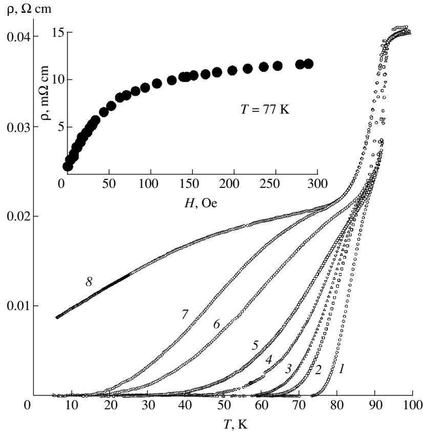
**Fig. 2.** Temperature dependences of the resistivity  $\rho$  of a 70 vol % YBCO + 30 vol % CuO composite measured at various values of the applied magnetic field strength  $H = 0$  (1), 38 Oe (2), 79 Oe (3), 183 Oe (4), 1 kOe (5), 10 kOe (6), 60 kOe (7) using a probing current density of 50 mA/cm<sup>2</sup> and  $H = 60$  kOe (8) using a probing current density of 0.5 A/cm<sup>2</sup>. The inset gives the plot of  $\rho$  versus  $H$  at  $T = 77$  K.
