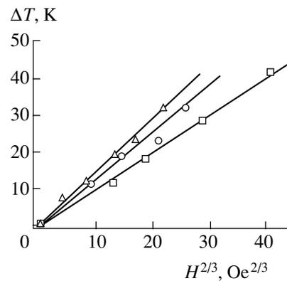
**Fig. 3.** The plots of  $\Delta T_c = T_c(H, R = 0) - T_c(H = 0, R = 0)$  versus  $H^{2/3}$  for various HTSC composites: (squares) 85 vol % YBCO + 15 vol % BaPbO<sub>3</sub>; (triangles) 85 vol % YBCO + 15 vol % CuO; (circles) 70 vol % YBCO + 30 vol % CuO.
