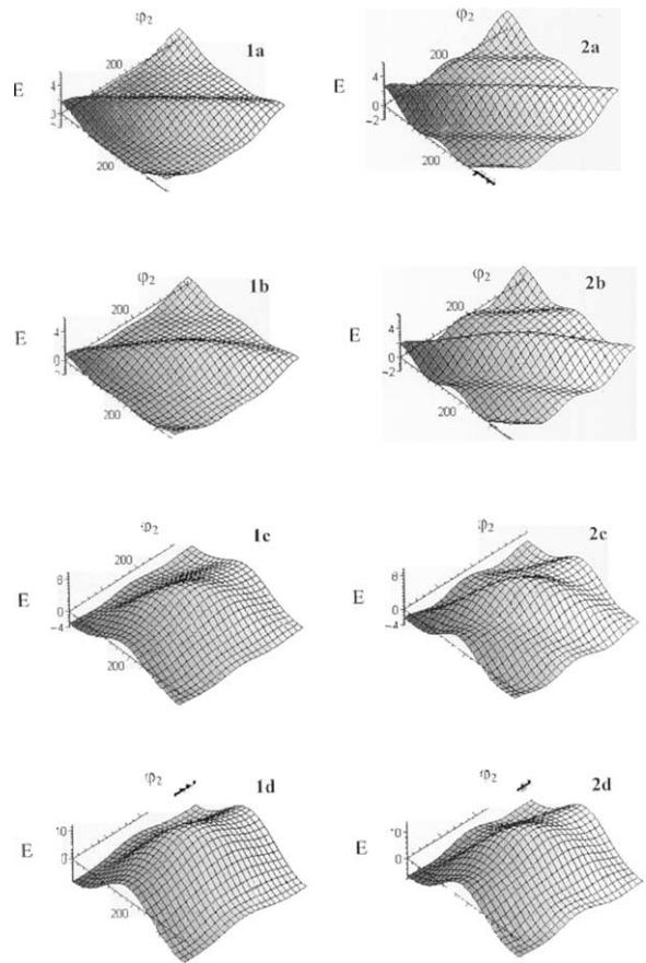
Fig. 4. Surfaces of the magnetic energy ( $E$ ) depending on the angles of magnetizations in layers  $\varphi_1$  and  $\varphi_2$ . Column 1:  $\eta = 0.7$ . Column 2:  $\eta = 1.7$ . (a)  $H = 5 \text{ Oe}$ , (b)  $50 \text{ Oe}$ , (c)  $300 \text{ Oe}$ , (d)  $600 \text{ Oe}$ .
