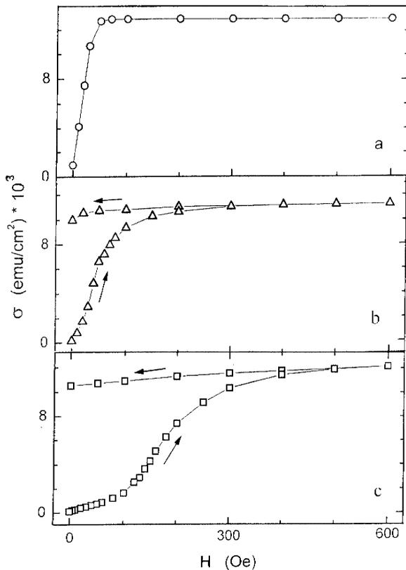
Fig. 3. Field dependences of the magnetization of the films (a)  $t_{Si} = 2 \text{ \AA}$ , (b)  $t_{Si} = 5 \text{ \AA}$ , (c)  $t_{Si} = 10 \text{ \AA}$ . Cooling conditions—ZFC.  $T = 4.2 \text{ K}$ . Arrows indicate directions of the temperature variation.
