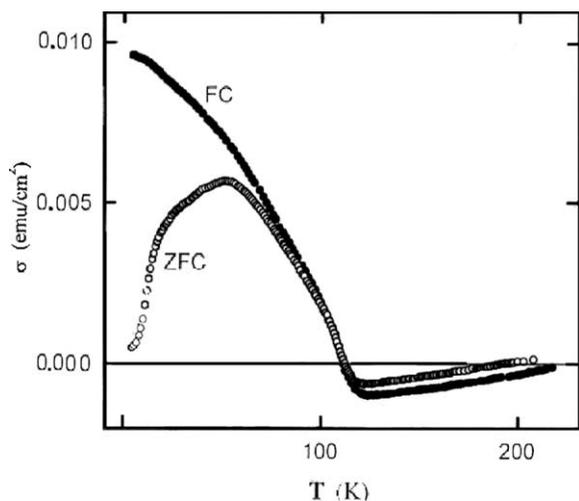
Fig. 1. Temperature dependences of the magnetization of the film with  $t_{\text{Si}} = 10 \text{ \AA}$  received with heating. FC: cooling regime  $H \neq 0$ , ZFC: cooling regime  $H = 0$ . The field of cooling and measuring is  $H = 20 \text{ Oe}$ .
