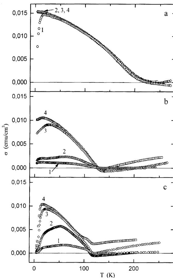
Fig. 2. Temperature dependences of the magnetization of the films received with heating. Cooling conditions—(ZFC). (a)  $t_{\text{Si}} = 2 \text{ \AA}$ , (b)  $t_{\text{Si}} = 5 \text{ \AA}$ , (c)  $t_{\text{Si}} = 10 \text{ \AA}$ . Curves 1, 2, 3, 4 are obtained in fields  $H = 10, 20, 50, 100 \text{ Oe}$ , respectively.
