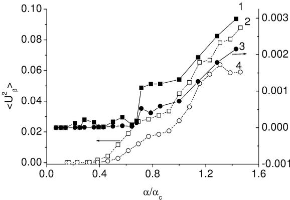
Fig. 2. Mean-square vibration  $\langle U^2 \rangle$  vs. spin–phonon coupling at  $\omega_0 = J$  (2,4),  $\omega_0 = 6J$  (1,3) along [10] (1,2,  $\beta = x$ ), [01] (3,4,  $\beta = y$ ) directions.
