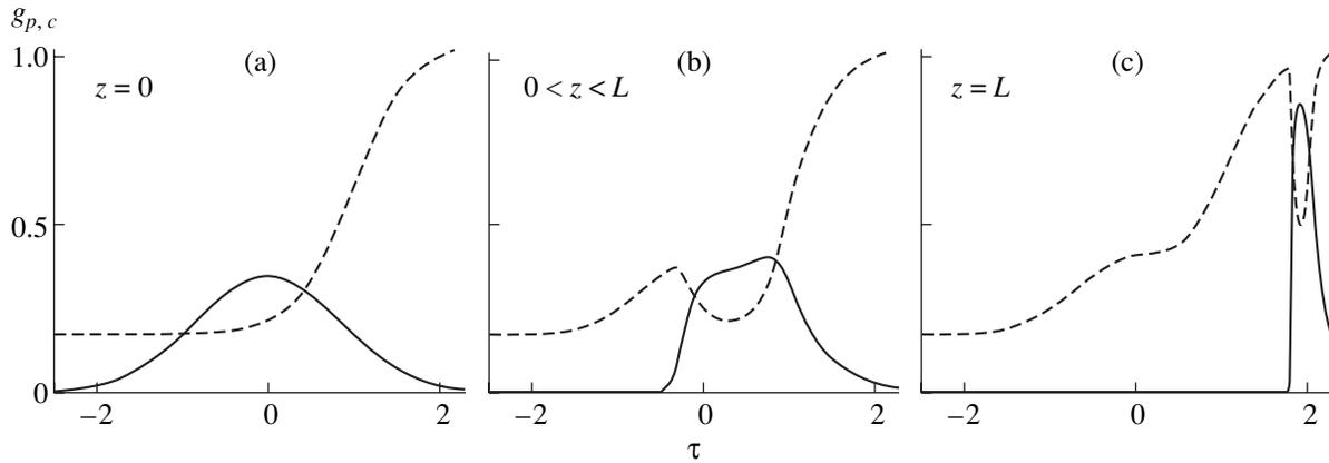
**Fig. 2.** Time profile of normalized Rabi frequencies for the probe pulse  $g_p = \frac{G_p(\tau)}{G_{\max}}$  ( $G_{\max}$  is the maximum value of the effective Rabi frequency) and coupling pulse  $g_c = \frac{G_c(\tau)}{G_{\max}}$  (dashed curve) in the case of different values of  $z$  coordinates inside the medium: (a) at the input of the medium,  $z = 0$ ,  $G_p(\tau = 0, z = 0) T_p = 20$ ; (b) at a certain distance  $z$ ; and (c) at the output of the medium,  $z = L$ .
