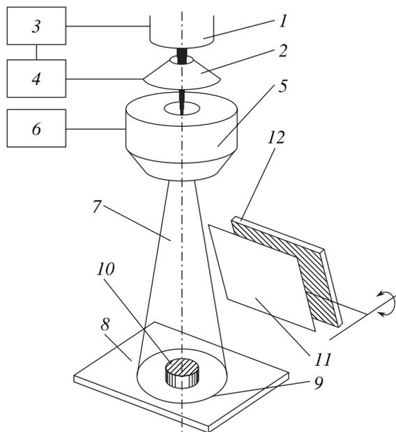
**Fig. 1.** Schematic diagram of the experimental arrangement: (1) plasma electron gun; (2) accelerating electrode; (3) discharge current source; (4) high-voltage source; (5) electromagnetic lens; (6) electron beam control unit; (7) annular electron beam; (8) graphite collector; (9) electron beam projection; (10) fullerene disk target; (11) shutter; (12) substrate.
