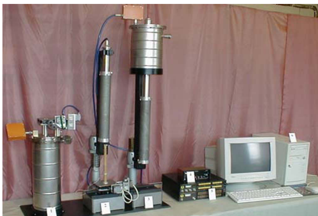
Figure 2. External view of a magnetic microscope (MM). From left to right are shown: 1- measuring channel with SQUID for "cold" objects study; 2- measuring channel with fluxgate for "warm" objects study; 3-measuring channel with SQUID for "warm" objects study; 4- scanner driving device; 5-SQUID and fluxgate electronic amplifier; 6- personal computer.
