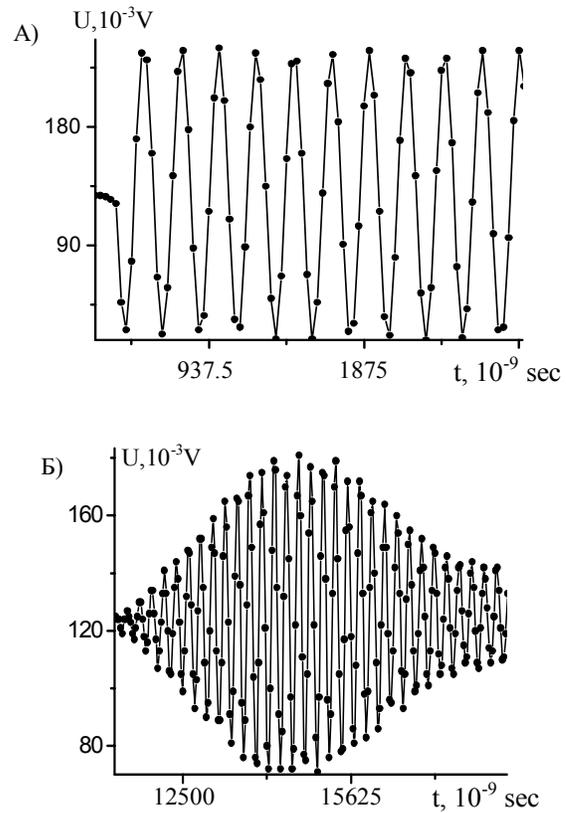
Figure 2. Example of a sound signal. (A) - registered by the first ADC channel; (B) - delaying in acoustic line and registered by the second ADC channel. Points mark out values of signal amplitude recorded in SRAM
