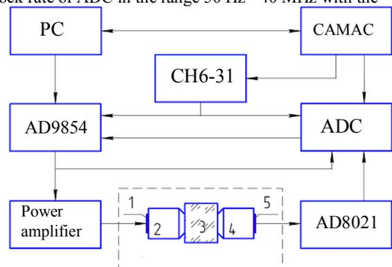
Figure 1. The block-scheme of automation pulse-phase method for acoustic measurings. 1, 5 - input and output piezoelectric transducers; 2, 4 - buffers; 3 - sample
