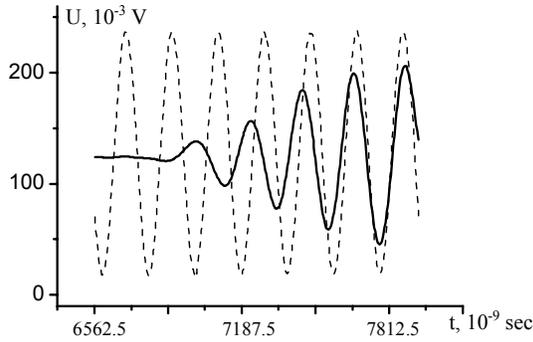
Figure 3. Effect of "signal tightening". The full curve - the delayed signal, the dashed - direct. Frequency of measuring is 5.1 MHz. The modification of frequency of the delayed signal is visible
