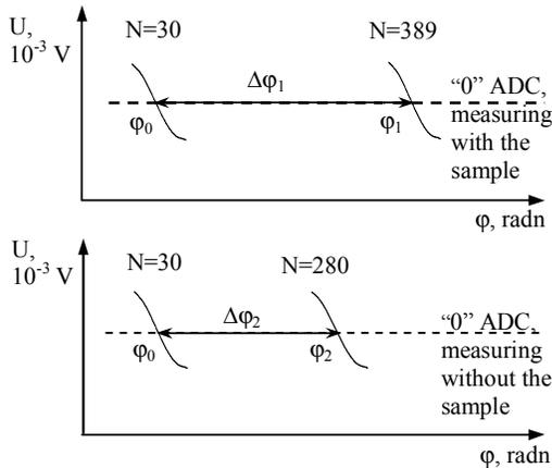
Figure 4. Definition of sound delay by the phase method
