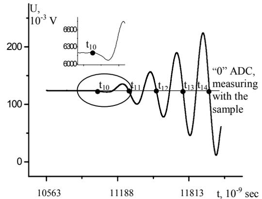
Figure 5. Measuring of sound delay by the method of the frequency strobing. Indicated time points  $t_i$  which are taken for evaluation  $V$ . On parenthesisizing - isolated the fragment of signal recorded with storage
