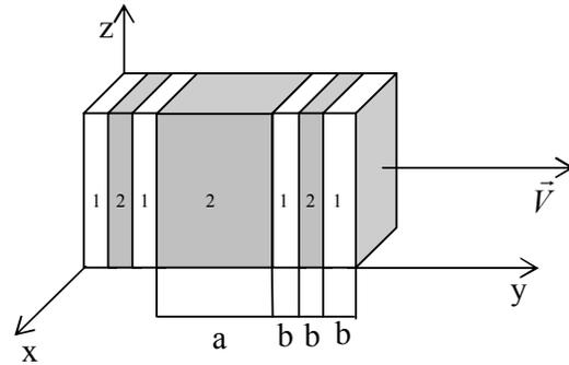
Figure 6. Structure of fractal type: 1 - acrylic plastic; 2 - Si. a = 3 mm, b = 1mm
