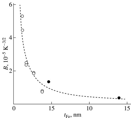
**Fig. 3.** Dependence of the Bloch constant  $B$  for  $(\text{Fe/Si})_n$  multilayer films on the thickness of the Fe individual layer. Open circles indicate the data obtained in this work, and closed circles correspond to the data taken from [14].
