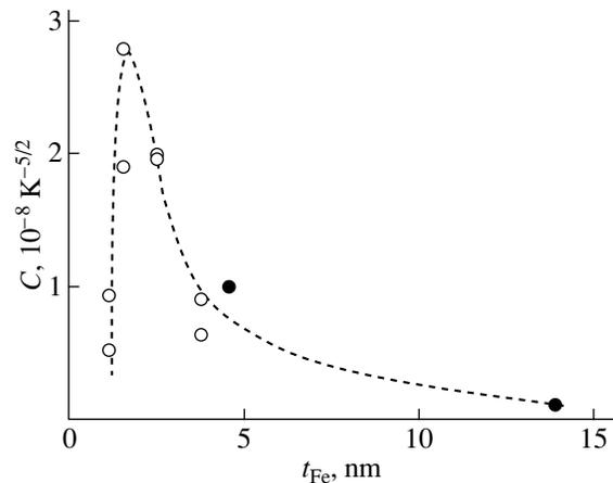
**Fig. 4.** Dependence of the constant  $C$  for  $(\text{Fe/Si})_n$  multilayer films on the thickness of the Fe individual layer. Open circles indicate the data obtained in this work, and closed circles correspond to the data taken from [14].
