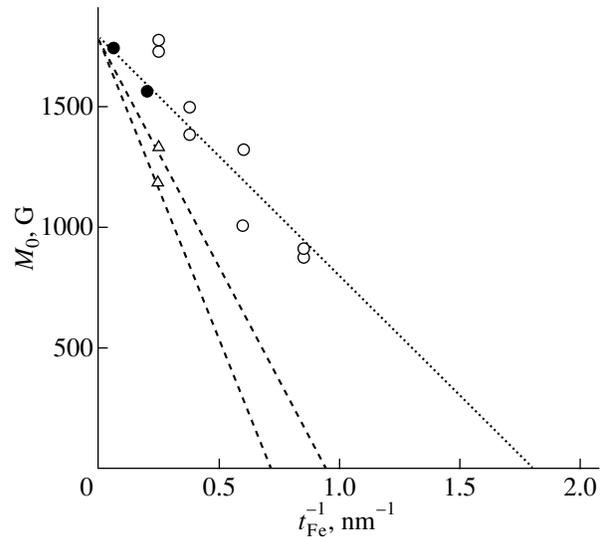
Fig. 6. Dependence of the experimental magnetization for  $(\text{Fe/Si})_n$  multilayer films on the quantity  $t_{\text{Fe}}^{-1}$ . Open circles indicate the data obtained in this work, closed circles correspond to the data taken from [14], and triangles represent the data taken from [20].
