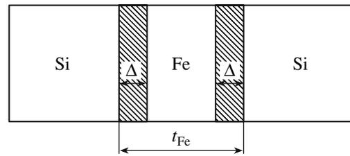
Fig. 5. Magnetic heterophase model of the  $(\text{Fe/Si})_n$  system.
