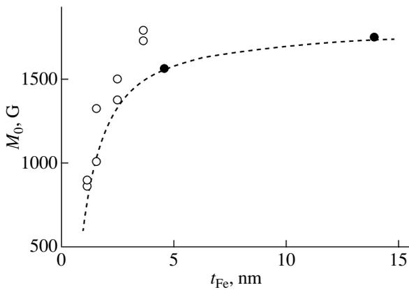
**Fig. 2.** Dependence of the magnetization  $M_0$  for  $(\text{Fe/Si})_n$  multilayer films on the thickness of the Fe individual layer. Open circles indicate the data obtained in this work, and closed circles correspond to the data taken from [14].
