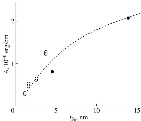
Fig. 7. Dependence of the exchange interaction constant  $A$  for  $(\text{Fe/Si})_n$  multilayer films on the thickness  $t_{\text{Fe}}$  of magnetic layers according to calculations from formula (4). Open circles indicate the data obtained in this work, and closed circles correspond to the data taken from [14].
