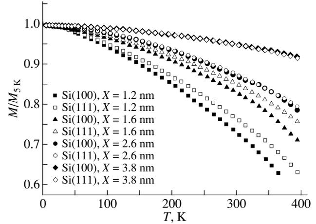
Fig. 1. Temperature dependences of the normalized saturation magnetization  $M/M_{5\text{K}}$  for  $(\text{Fe}/\text{Si})_n$  multilayer films at different thicknesses of  $\text{Fe}(X)$  individual layers.
