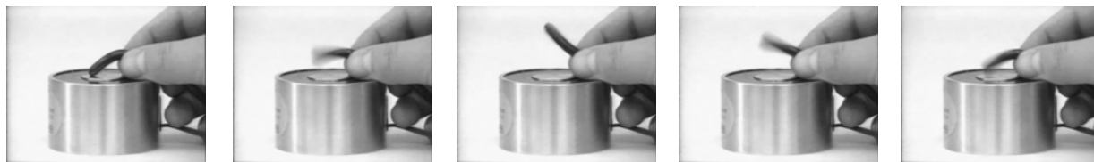
Fig. 1 Snapshot of shape change of a magnetite-loaded PDMS elastomer due to modulated magnetic field. The frequency of the field is 40 Hz.
