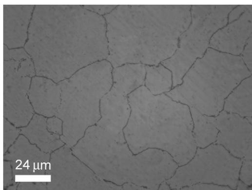
Fig. 5. Austenitic structure, usual for  $\text{Fe}_{86}\text{Mn}_{13}\text{C}$  in an initial condition before loading.
