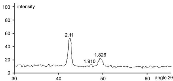
**Fig. 7.** Diffraction picture of X-ray received from a surface of  $\text{Fe}_{86}\text{Mn}_{13}\text{C}$  sample, from an austenitic grain.
