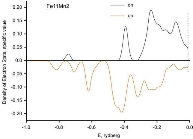
**Fig. 9.** Density of spin-polarized electronic conditions of a chosen nanocluster FK12, received by self-consistent field method.
