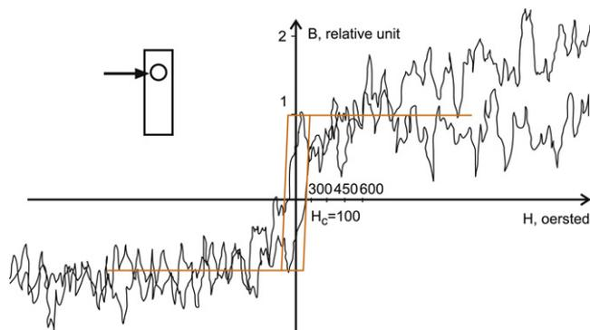
Fig. 4. Measurement of coercive force in marked area for bulk sample (Fig. 1).
