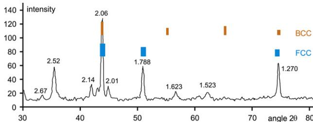
**Fig. 8.** Diffractogram of  $\text{Fe}_{86}\text{Mn}_{13}\text{C}$  received from intergranular layers, at scanning a sample's surface by X-ray beam.
