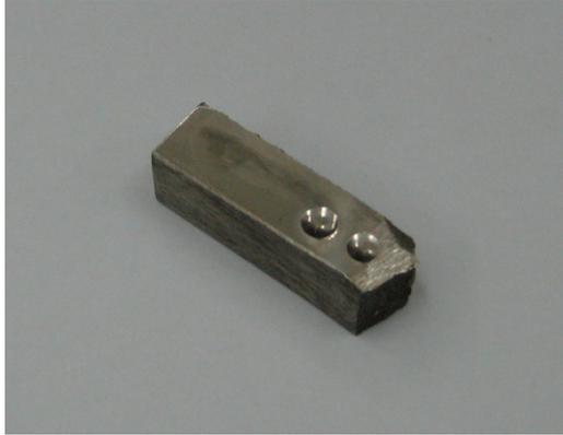
**Fig. 1.** The Illustration of  $\text{Fe}_{86}\text{Mn}_{13}\text{C}$  sample after dynamic loading 3000 kg on installation of test of hardness by Brinell's method.
