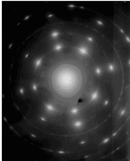
**Fig. 2.** The picture of electron diffraction, received from thin film sample of Fe–Mn–C, of two-dimensional quasicrystal which also have an eight-fold symmetry axis.
