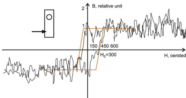
**Fig. 3.** Measurement of coercive force far from marked area for bulk sample (Fig. 1).
