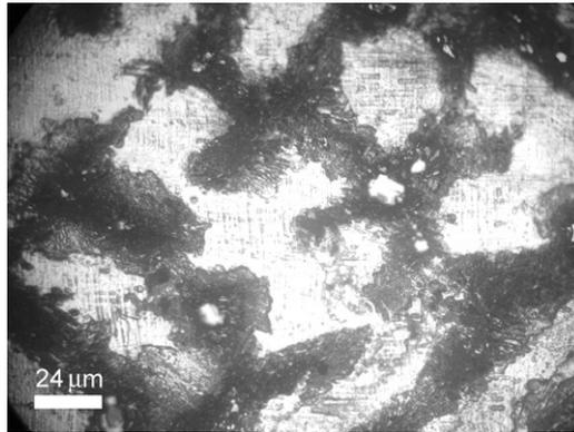
**Fig. 6.** Structure of samples after long shock stressing in an operating mode of rock-crushing machine (the wide dark layers have appeared between light grains of austenite).
