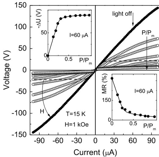
**Figure 2.**  $V$ – $I$  curves of the structure for different power densities of optical radiation (980 nm) at 15 K and  $H = 1$  kOe;  $P/P_m$  and  $P_m$  are the same as in figure 1; dashed curve is a dependence for  $H = 0$  and  $P = 0$ . The top inset shows the dependences of the photovoltaic effect on power density. The bottom inset shows the dependence of the MR on power density.
