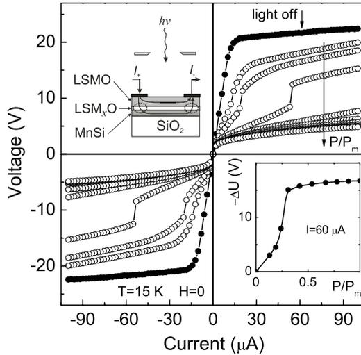
**Figure 1.**  $V$ - $I$  curves of the structure for different power densities of optical radiation (980 nm) at 15 K without a magnetic field;  $P/P_m = 0.13, 0.19, 0.24, 0.31, 0.42, 0.54, 0.67, 0.78, 0.89$  and  $1$ ;  $P_m = 60 \text{ mW cm}^{-2}$ . The top inset schematically illustrates the tunnel structure and photovoltaic measurement geometry; the arrow curves show the possible current channels. The bottom inset shows the dependences of the photovoltaic effect on power density.
