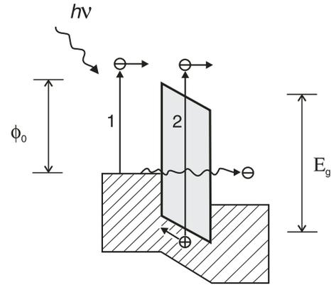
**Figure 3.** Schematic band diagram of the tunnel junctions in the structure and two possible mechanisms of the photovoltaic effect: (1) photoemission of the electrons from the metal electrode; (2) generation of the electron–hole pair due to the interband absorption in the dielectric layer.
