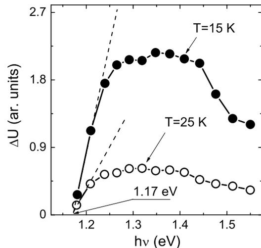
**Figure 4.** Dependences of the photovoltaic effect on photon energy  $h\nu$  at 15 and 25 K.
