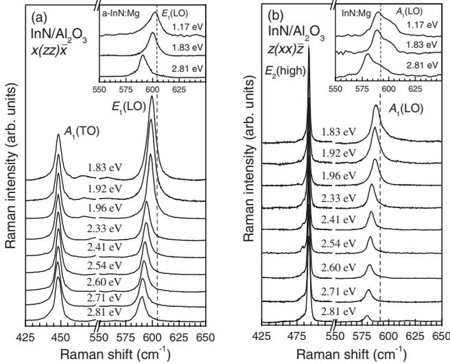
FIG. 1. Room-temperature polarized Raman spectra of  $E_1(\text{LO})$  and  $A_1(\text{LO})$  modes of hexagonal InN obtained in  $x(\text{zz})\bar{x}$  and  $z(\text{xx})\bar{z}$  scattering configurations for different excitation energies. Here,  $z$  is the InN hexagonal axis direction. The dashed lines show estimated LO phonon frequencies at the  $\Gamma$  point.
