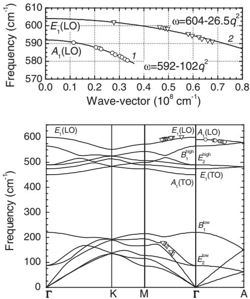
FIG. 3. Top panel: frequencies of  $A_1(\text{LO})$  and  $E_1(\text{LO})$  phonons as a function of phonon wave vectors  $q=2p_\omega$ . The wave vectors are calculated for E-LH (curve 1) and E-HH (curve 2) transitions. The symbols are experimental frequencies. The solid lines are dispersion approximations of  $A_1(\text{LO})$  and  $E_1(\text{LO})$  branches by parabolic curves. Lower panel: InN phonon-dispersion curves taken from Ref. 15 and experimental data of this work (symbols).
