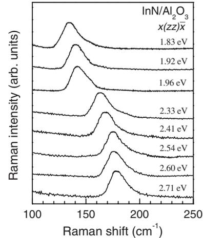
FIG. 4. Room-temperature polarized Raman spectra of hexagonal InN in the region of acoustic phonons obtained in  $x(zz)\bar{x}$  scattering configuration for different excitation energies. Here,  $z$  is the InN hexagonal axis direction. The spectra are normalized to the Raman line maximum.
