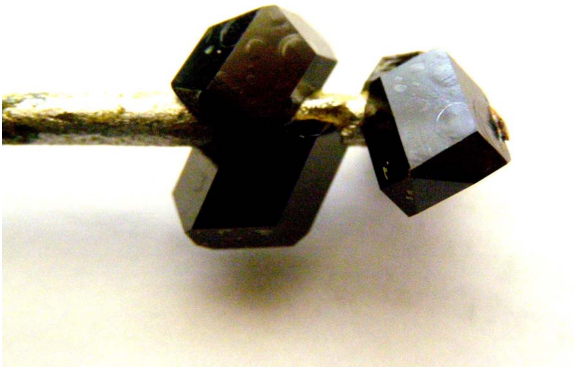
Fig. 1. \text{Nd}_{0.75}\text{Dy}_{0.25}\text{Fe}_3(\text{BO}_3)_4 single crystal grown from bismute molibdate based flux.
