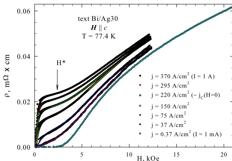
**Fig. 7** The magnetoresistance  $R(H)$  of sample text Bi/Ag0 ( $\mathbf{H} \parallel c$  configuration) at 77.4 K for various current densities (pointed in the figure). The field  $H^*$  corresponded to change of curvature of  $R(H)$  dependences is pictured
