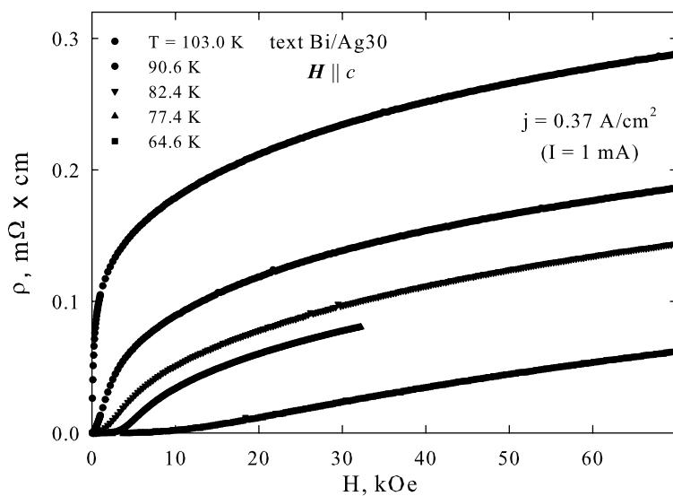
**Fig. 5** The resistive transition under various magnetic fields of polycrystalline BSCCO. *Insert:* the same for the field range  $0 \div 10^3$  Oe. *Horizontal arrow* indicates possible resistive response from IGBs for data at  $H$  lower than  $10^2$  Oe
