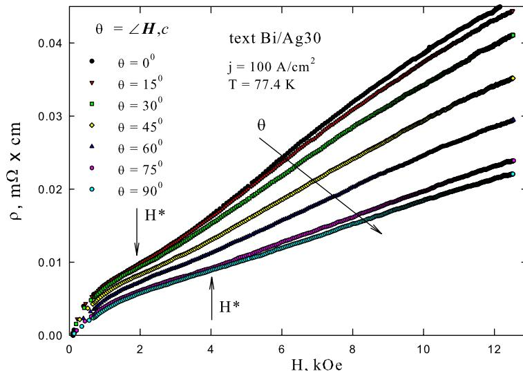
**Fig. 9** The magnetoresistance of sample poly-Bi at 77.4 K for various current densities (pointed in the figure)
