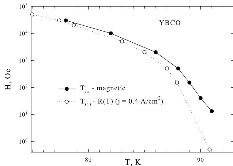
**Fig. 11** The irreversibility line  $H_{\text{irr}}(T)$  (obtained from magnetic measurements) and the dependences  $T_{C0}(H)$  obtained from measurements of  $R(T)$  and  $R(H)$  at various transport currents (*pointed* in the figure) in coordinates  $H$ ,  $T$  (semilog scale) of sample text Bi/Ag30. For details, see the text
