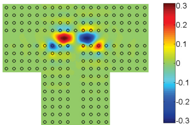
FIG. 2. (Color online) (Color online) The solution of Maxwell equations for the case shown in Fig. 1(a) which demonstrates the antisymmetric FPI BSC (antisymmetric standing wave between nonlinear off-channel defects marked by stars) with frequency \omega_c a / 2\pi c = 0.3402 . Only that part of the PhC is shown where the scattering wave function \Psi_S is given in the Lippmann-Schwinger Eq. (2).
