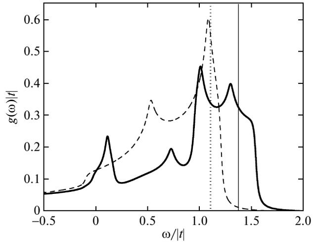
**Fig. 3.** Density of states calculated in the Hubbard-I approximation (dashed line) and also calculated taking into account the spin and charge fluctuations (thick solid line). Comparing the density at the intersection point of the dotted and dashed lines and the density at the intersection point of the thin and thick lines, one can see that the inclusion of the fluctuations leads to a strong decrease in the density of states in the vicinity of the Fermi level.
