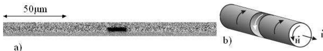
Fig. 1. Foto (a) and schematic picture (b) of single circular domain in microwire.
