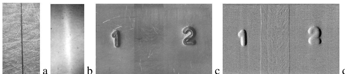
Fig. 1. Surface (a) and MO EC image (b) of 10 \mu m slot in thin Al plate (stroboscopic mode); surface and MO EC image of defect-free welded joint in thick Al plate (magnetographic mode).
