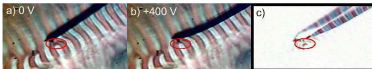
Figure. Displacement of the domain walls a) Original position b) Displacement under the influence of an electric field c) difference image.
