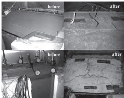
Fig. 2. Surface condition of the roadbeds before and after the cyclical freeze-thaw ( upper left : roadbed with Lanzhou loess before the experiment; upper right : roadbed with Lanzhou loess after the experiment; lower left : roadbed with Lanzhou loess injected sulfate sodium solution before the experiment; lower right : roadbed with Lanzhou loess injected sulfate sodium solution after the experiment).
