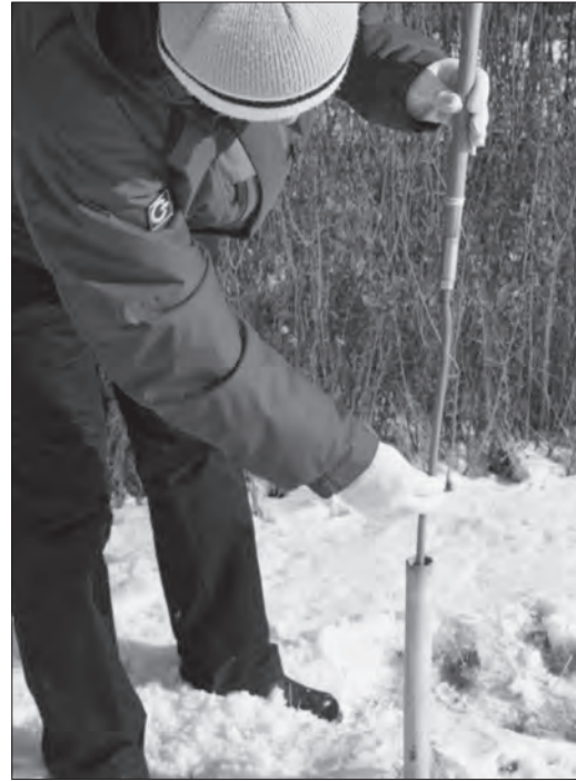
Fig. 4. Manual measurement of freezing depth with Danilin freezing depth device.
