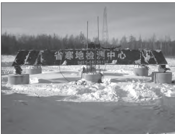
Fig. 3. Vertical steady pulling of separate pile.
