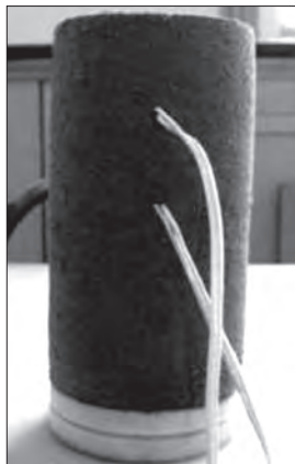
Fig. 1. Specimen with two thermistor temperature sensors.
