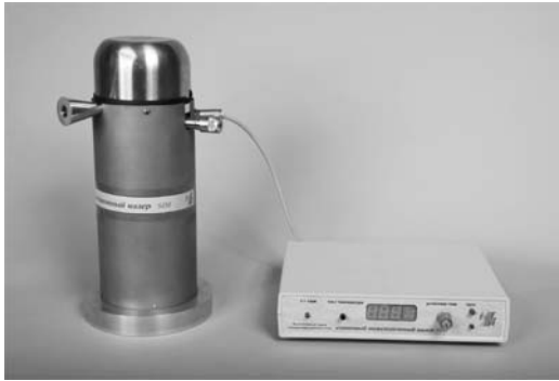
Fig. 1. The mock-up of a solid-state quantum generator (maser) with spin-polarized electrons injection.
