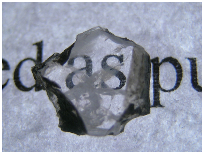
Fig. 1. Photo of K_3WO_3F_3 single crystal on the background of Times Roman font 12.
