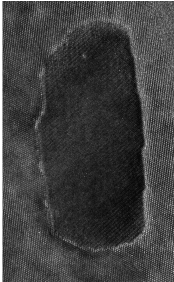
Fig. 4. Transmission electron microscopy photo of the \beta -FeSi 2 particle embedded in the silicon matrix.
