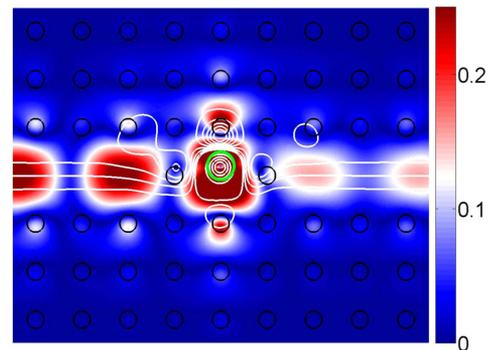
Fig. 3. (Color online) Absolute value of light amplitude (electric field) and optical streamlines (white lines) in the PhC waveguide with single nonlinear defect shown by gray open circle for  $a\omega/2\pi c = 0.36$ ,  $P = 10 \text{ W}/a$ ,  $\theta = 0$ .
