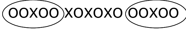
Fig.3 Phase-separated state at the densities \frac{1}{2} - \delta_C < n_{el} < \frac{1}{2} with nano-scale metallic clusters inside CO checkerboard insulating matrix for V \gg t .
