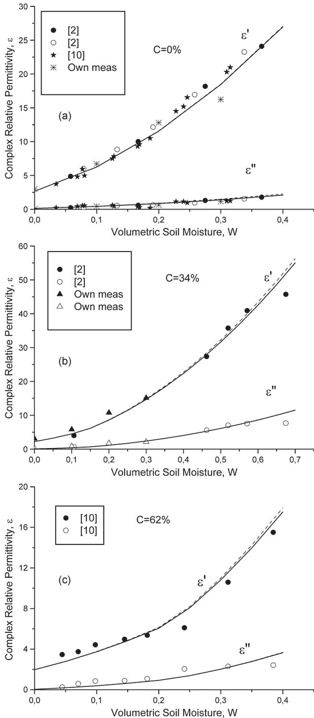
Fig. 1. Measured and calculated CRPs  $\epsilon = \epsilon' + i\epsilon''$  for the soils with different clay contents at room temperature (20 °C): (a)  $C = 0\%$ , (b)  $C = 34\%$ , and (c)  $C = 62\%$ . Measured data are taken from [2] and [10] and obtained by the authors (own measurement). Dielectric calculations with the model in [5] and monofrequent model are represented with solid and dashed lines, respectively.
