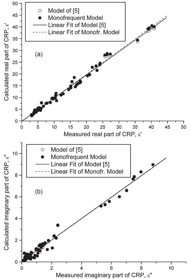
Fig. 3. Correlation of the measured (a) real part  $\epsilon'$  and (b) imaginary part  $\epsilon''$  of CRP with the calculated ones obtained by using the model in [5] and monofrequent model, respectively.
