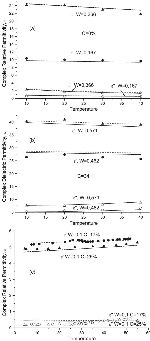
Fig. 2. Measured and calculated CRPs as functions of temperature for soils with different clay contents  $C$  and soil moistures  $W$ : (a)  $C = 0\%$ , (b)  $C = 34\%$ , and (c)  $C = 17\%$  and  $25\%$ . Measured data are taken from [2] and obtained by the authors. Dielectric calculations with the model in [5] and monofrequent model are represented with solid and dashed lines, respectively.
