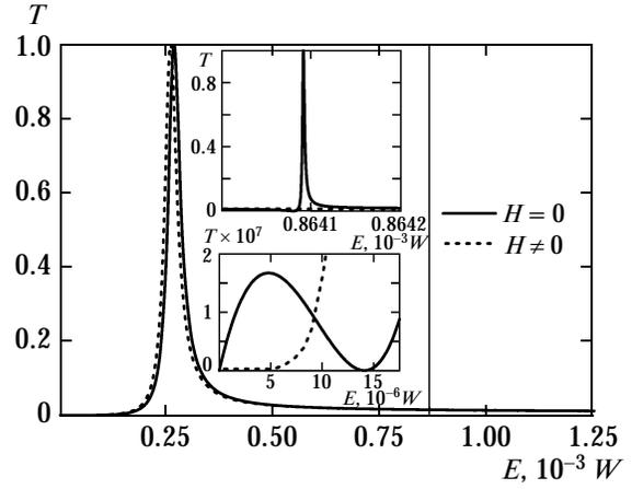
**Fig. 3.** Low-energy region of the dependence  $T(E)$  upon transport through a spin dimer,  $t = -1$  eV,  $\tau = 0.075$ ,  $J = A = 1.25 \times 10^{-3}$ ,  $\mu_B H = 1.25 \times 10^{-4}$ ,  $\varepsilon_D = -0.498$ ,  $g = 1.88$ . The structure of the induced asymmetric peak is shown in the upper inset. The shift of the antiresonance with energy  $E_{ares1}$  in a magnetic field is shown in the lower inset.
