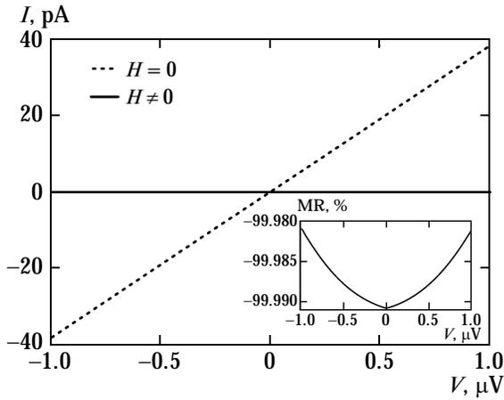
**Fig. 4.** Current–voltage characteristic of a system with a magnetic impurity for the parameters of Fig. 2,  $E_F = 0.115 \times 10^{-3}$ . The system’s magnetoresistance is shown in the inset.
