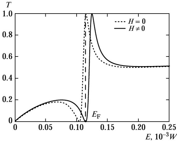
**Fig. 2.** Low-energy region of the dependence  $T(E)$  for the tunneling coupling of a magnetic impurity to the electrodes,  $t = -1$  eV,  $\tau \approx 0.25$ ,  $\varepsilon_D \approx -0.47$ ,  $D = A = 0.25 \times 10^{-3}$ ,  $\mu_B H = 1 \times 10^{-4}$ ,  $g = 1$ .
