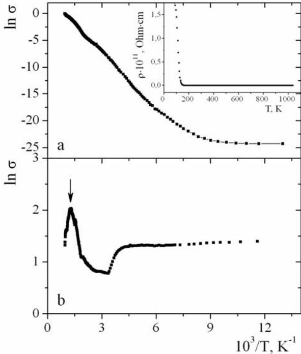
Fig. 3. Temperature dependences of conductivity for the  $Mn_{1-X}Ni_XS$  samples with  $X = 0.05$  (a) and  $X = 0.1$  (b).
