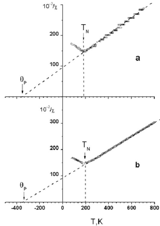
Fig. 2. Temperature dependences of the magnetic susceptibility for  $Mn_{0.95}Ni_{0.05}S$  (a) and  $Mn_{0.9}Ni_{0.1}S$  (b) samples measured in the magnetic field 8,6 kOe.
