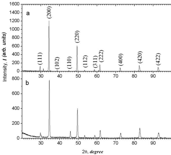
Fig. 1. X-ray diffraction patterns of  $Mn_{0.95}Ni_{0.05}S$  (a) and  $Mn_{0.9}Ni_{0.1}S$  (b) samples measured at  $T = 300$  K before heat treatment.
