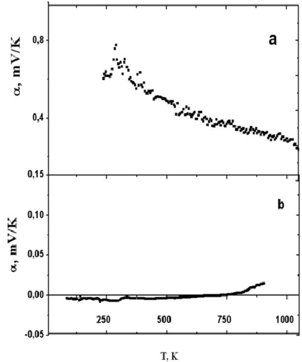
Fig. 4. Temperature dependences of thermopower coefficient for  $Mn_{1-X}Ni_XS$  samples with  $X = 0.05$  (a) and  $X = 0.1$  (b).
