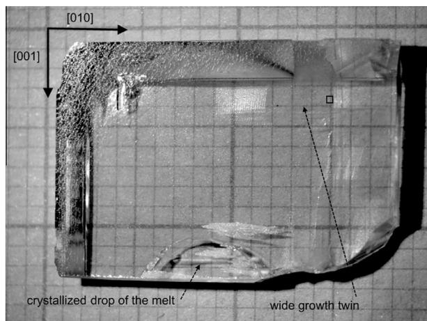
**Fig. 2.** Bottom growth facet  $(100)$  of the PBO crystal after etching.
