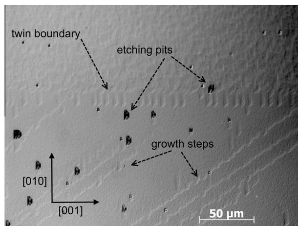
**Fig. 3.** Etched bottom  $(100)$  growth facet of the PBO crystal (square-marked in Fig. 2).
