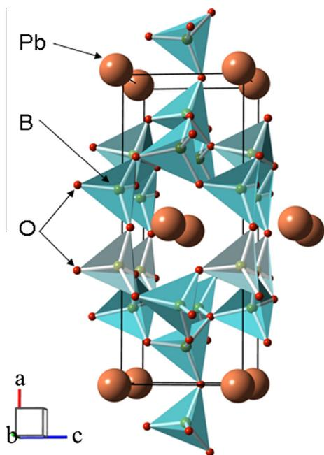
**Fig. 1.**  $\text{PbB}_4\text{O}_7$  crystal structure. The unit cell is outlined. Lone boron and oxygen atoms are omitted for clarity.
