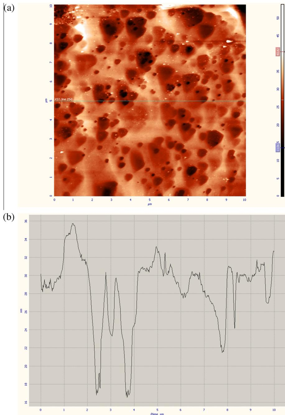
Fig. 6. AFM pattern recorded from (100) etched surface: (a) panoramic view and (b) depth profile.
