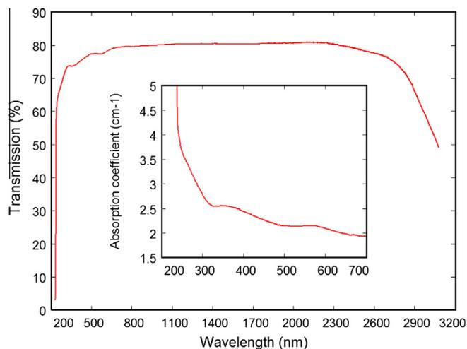
**Fig. 4.** Unpolarized transmission spectrum of PBO crystal in the direction of  $(100)$  axis. Inset: absorption in the UV and visible ranges.
