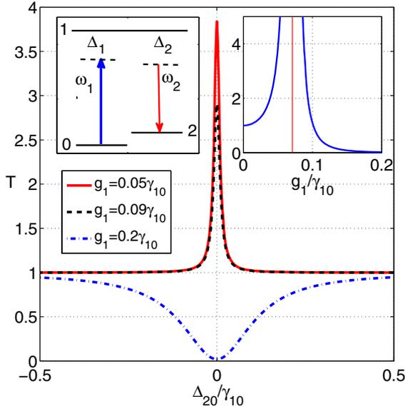
Fig. 1. Transmission spectra  $T$  of PhC with Raman gain defect as a function of detuning from the Raman resonance ( $\omega_2$  changes at  $\Delta_1 = 30\gamma_{10}$ ) for various Rabi frequencies  $g_1$  at the input of PhC. Left inset: energy-level diagram of a three-level atom in a Raman gain scheme. Right inset: transmission coefficient for a probe field versus Rabi frequency of a pump  $g_1$ . The vertical line refers to the threshold value of  $g_1$ .
