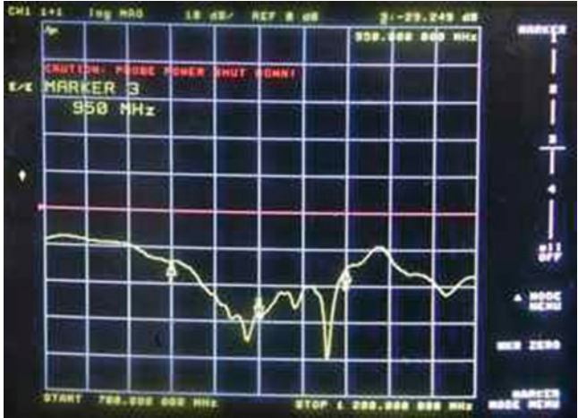
Fig. 19.13 Measured return loss of the RFID antenna
